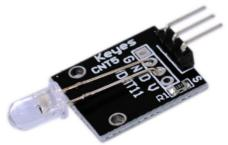
The LED 7 Color Flashing Module incorporates a 5mm tri-color (RGB) LED
