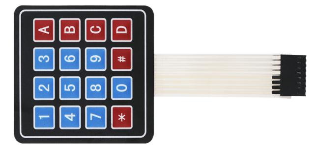
Beneath each key is a membrane switch. Each switch in a row is connected to the other switches in the row by a conductive trace underneath the pad. Each switch in a column is connected the same way – one side of the switch is connected to all of the other switches in that column by a conductive trace. Each row and column is brought out to a single pin, for a total of 8 pins on a 4X4 keypad:
