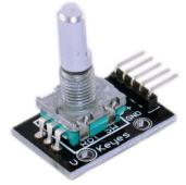
A rotary encoder is a type of position sensor that converts the angular position
