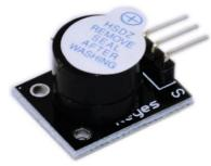
The Active buzzer is the simplest sound making module. You can use high/low
