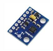
MMA8452Q is a smart low-power, three-axis, capacitive micromachine acceleration
