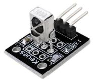
The KY-022 Infrared Receiver module reacts to 38kHz IR light. It can be used to receive commands from IR remote controllers from TVs, stereos and other devices.
