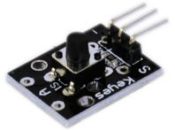
This is a basic button module. You can simply plug it into an IO shield to have your first try of Arduino. The KY-004 Key Switch Module is a push button that will close the circuit when pressed, sending a high signal.
