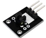
The KY-010 Photo Interrupter module is a switch that will trigger a signal when light between the sensor's gap is blocked. It is used for many applications including optical limit switches, pellet dispensing, general object detection, etc.
