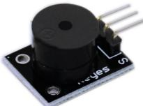
The buzzer we introduced here is a passive buzzer. It cannot be actuated by itself, but by external pulse frequencies. Different frequencies produce different sounds. You can use Arduino to code the melody of a song, quite fun and simple.
